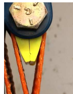
Both legs lie against each other and the bulge lies in the recess. The applied pretensioning force is 1000 daN.
