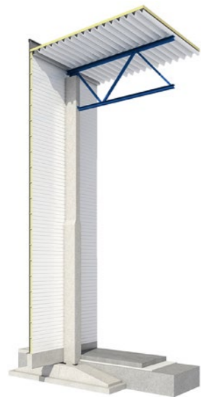
Reinforced concrete support with truss beams
